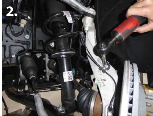
2. Remove brake sensor, brake line, and abs sensor from spindle. (10mm socket) (pic 2)
