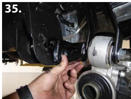
30. Install passenger sider differential drop bracket in to factory location using the factory hardware. DO NOT TIGHTEN YET. (pic 32)
