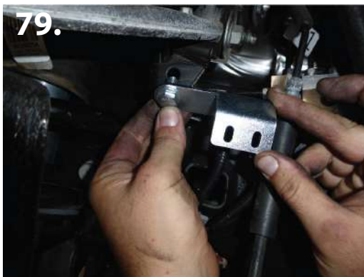
71. Install new abs sensor drop bracket located inside the hardware bag. (pic 79-80)
