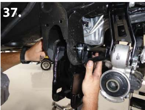
34. Install rear crossmember using provided 18mm x 120mm bolts. DO NOT TIGHTEN YET. (pic 36-37)
