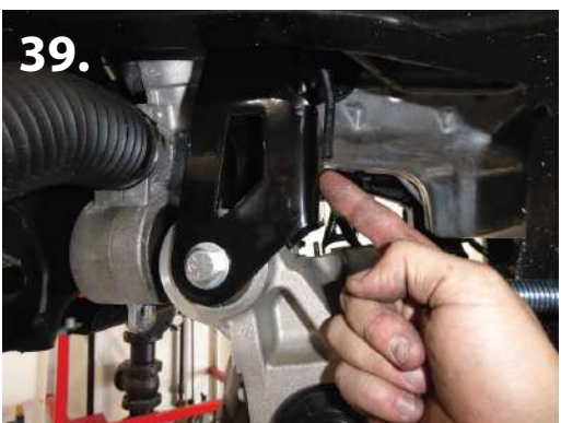
35. Use factory hardware to install differential on rear crossmember mount. (pic 38)
