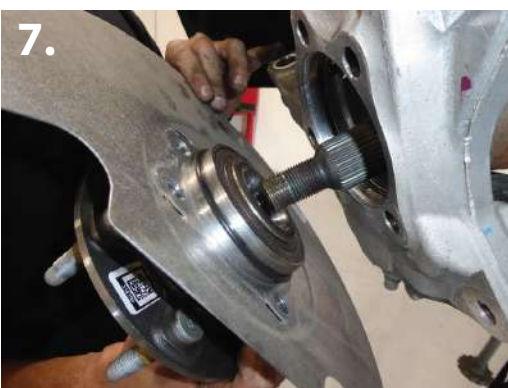
7. Remove hub assembly and dust shield. Hub has a seal, so it will be very snug. (pic 7)
