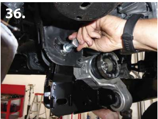
34. Install rear crossmember using provided 18mm x 120mm bolts. DO NOT TIGHTEN YET. (pic 36-37)
