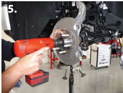
4. Remove rotor and CV axle nut. (36mm socket) (pic 5)
