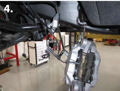
4. Remove rotor and CV axle nut. (36mm socket) (pic 5)
