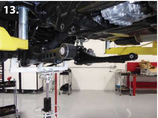
14. Remove the factory radius arms. Use a 27mm socket on the upper arm to axle bolts and a 24mm socket on the lower arm to axle bolts. Use a 27mm socket on the arm to frame bolts. (pic 13)
