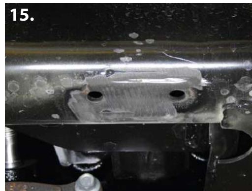
15. Use a cut-off wheel to remove the front bump stop mounts on both sides of the frame. The mounts will be reused, so do not destroy them. Cut the factory weld only. (pic 14)
