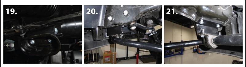
**15.** Install new front sway bar drop brackets using the provided 3/8" x 1" bolts. Install the factory sway bar mounts onto the new drop brackets using the factory hardware. (pic 20-21)
