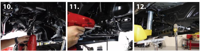
8. Unbolt the factory front track bar mount. Use a 21mm socket. (pic 10-11)
