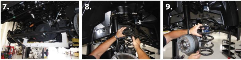
6. Slowly lower the front axle. Be sure to keep brake lines, abs lines, and the electronic 4wd cylinder wire (on passenger side) clear of any obstructions. Do not over extend the drive line. It can break or bend if dropped too far. Be careful not to let the front coils fall as you lower the axle. (pic 7)
