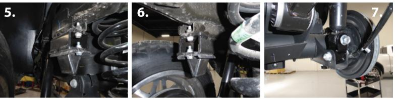
11. Install rear bump stop drop brackets using the provided 3/8" x 1-1/4" bolts. (pic 5-6)
