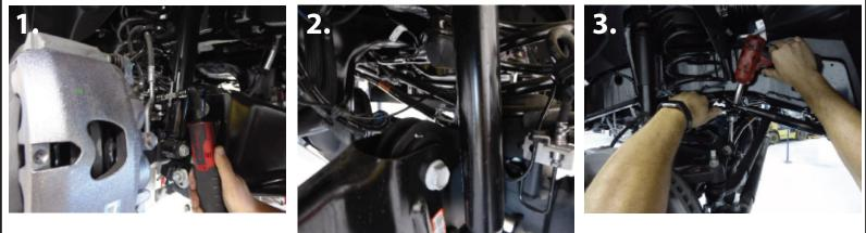
**1.** Disconnect the brake lines from the front axle on both sides. There will be four bolts total. Use a 13mm socket. (pic 1-2)
