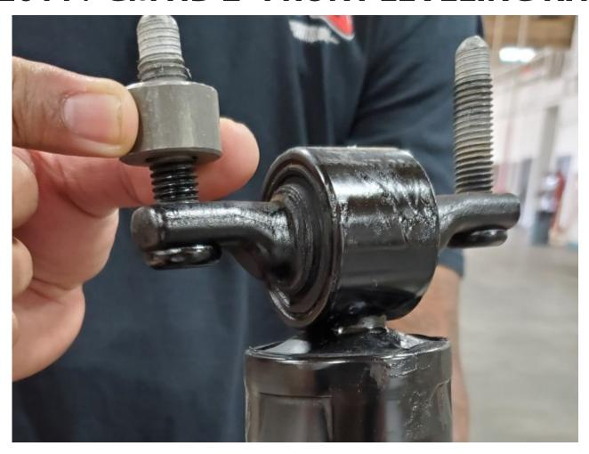
Use the four provided spacers and install on on each shock stud as shown in the picture. Use the new provided flange nuts to install the upper shock into the factory location and tighten to 50 ft lbs. Re-install the lower (bottom) end of the factory front shock into the factory position in the shock mount, using all the original hardware and tighten.
