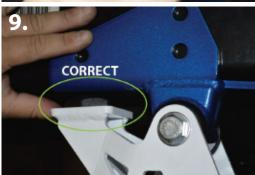
12. With the brackets fully assembled, lift the frame mount up and place against the bottom of the frame. Making sure there is no gap between the bump stop and the frame mount. (pic 8-9)
