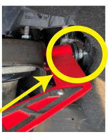
Also, do not forget to grease the ball joints after installing the new upper control arms.
