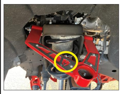
When installing the new McGaughy's upper control arms, the "M" badge will be towards the front of the vehicle. Use the new provided hardware to install the upper arms into the factory location. Make the washers are insatlled on the outside ends on the bushings of the new upper arms.
