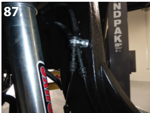
77. Use provided Adell clamp to connect abs and brake sensor wire to neck of spindle. Be sure to turn wheels both ways to make sure there is plenty of room and nothing is getting caught up. (pic 87)
