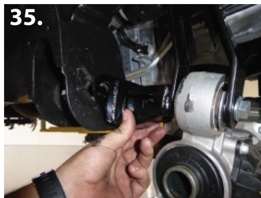
30. Install passenger side differential drop bracket in to factory location using the factory hardware. DO NOT TIGHTEN YET. (pic 32)
