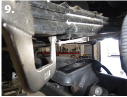
9. If your vehicle has a tapered shim under leafs, you must remove that shim. Clamp leaf pack together and remove center pin. Remove the tapered shim. (pic 9-10)
