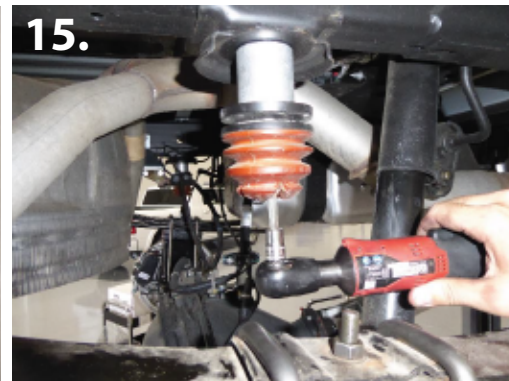
12. Remove factory bump stops. 13. Reinstall bump stops using new drop down spacers and allen bolts. (pic 14-15)
