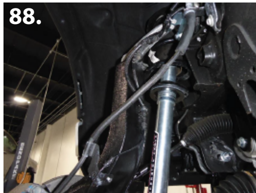
77. Use provided Adell clamp to connect abs and brake sensor wire to neck of spindle. Be sure to turn wheels both ways to make sure there is plenty of room and nothing is getting caught up. (pic 87)
