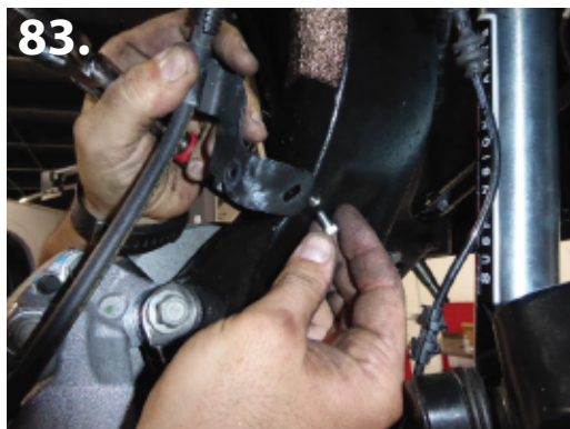
72. Remove factory bracket located lower on the abs sensor. This mount will no longer be used. (pic 81)
