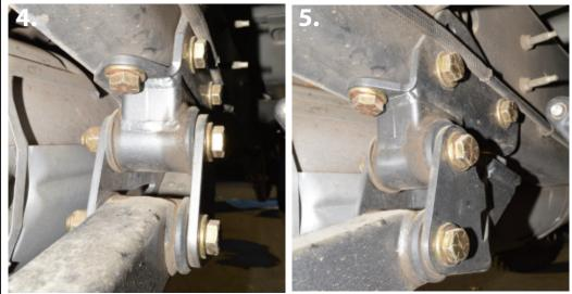
4. Assemble shackles and frame mount brackets with provided bump stops, bushings, and sleeves.
