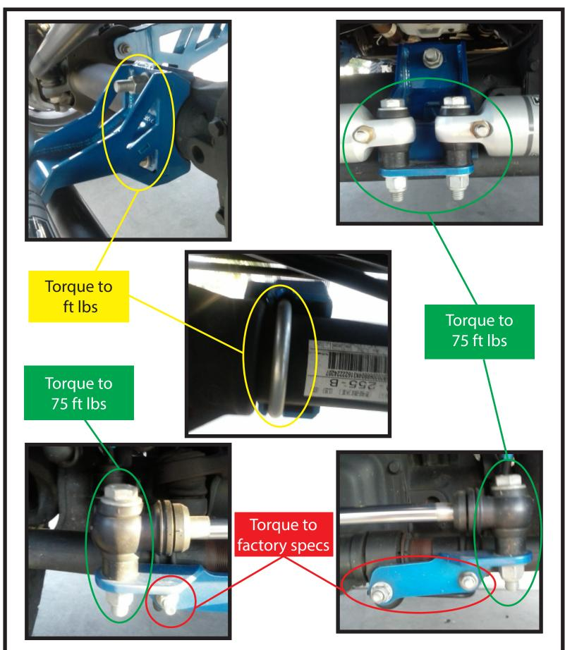
Be sure to go over all hardware and retorque after 500 miles. Kit was designed to use FOX SHOCKS part # 985-24-063. When installing shocks, make sure to turn the wheels all the way to the right and left. Make sure the shocks are not limiting the steering, or they will fail. McGaughy's warranty does not cover FOX SHOCKS or any factory components.
