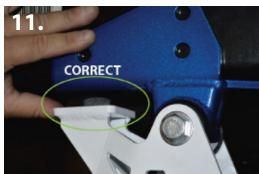
14. With the brackets fully assembled, lift the frame mount up and place against the bottom of the frame. Making sure there is no gap between the bump stop and the frame mount. (pic 10-11)
