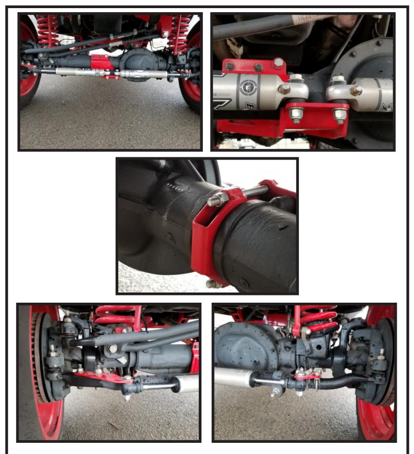
Be sure to go over all hardware and retorque after 500 miles. Kit was designed to use FOX SHOCKS part # 985-24-063. When installing shocks, make sure to turn the wheels all the way to the right and left. Make sure the shocks are not limiting the steering, or they will fail. McGaughy's warranty does not cover FOX SHOCKS or any factory components.
