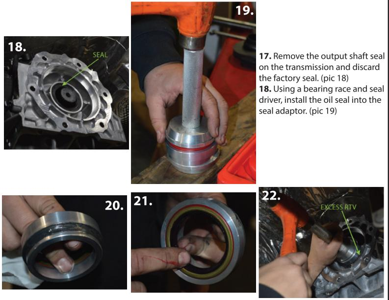
**19.** After the seal is installed, apply a small amount of RVT silicon to the seal adaptor. (pic 20) Also, apply a small amount of grease to the seal. (pic 21)
