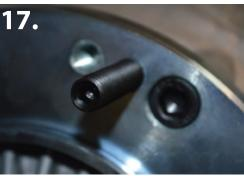
NOTE: Picture 16 shows in the **recommended** 20 degree position. You will need to install the McGaughy's transmission crossmember in this position. Picture 17 shows the 10 degree position, which can run the factory crossmember with trimming.
