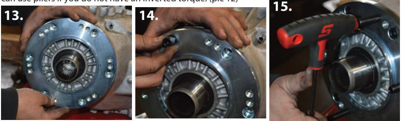
14. Take the index ring and locate the position where the bolt pattern matches up to the transfer case. (pic 13)
