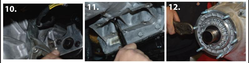
11. Remove the 3 Christmas tree clamps that hold the wire to the transfer case. (pic 10) And disconnect the vent tube using pliers.
