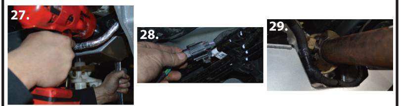
**26.** Install the McGaughy's crossmember with the large cut out on the driver side, using the factory hardware and a metric 24 wrench. (pic 27)
