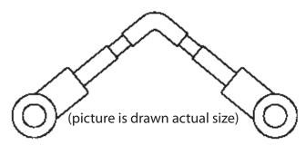
Lay your rod on top of picture to make sure the bend is the same, it should match.
