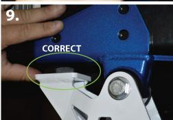
12. With the brackets fully assembled, lift the frame mount up and place against the bottom of the frame. Making sure there is no gap between the bump stop and the frame mount. (pic 8-9)
