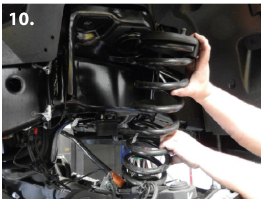
11. Slowly lower the front axle until the front coil spring tension is released.
