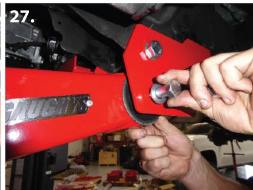
**27.** Reinstall the radius arm drop brackets over the original mount. Install the sleeve spacer and use 18mm x 130mm bolt to mount. Now use the provided 1/2"-13 x 1-1/4" bolts into the rivet nuts installed into the frame. Torque these two bolts first, to 70 lbs. Next torque the bolt going through the sleeve to 90 lbs. (pic 25-26)
