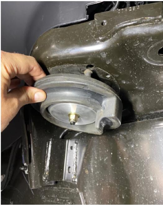
3. With the backing plate installed, slide the supplied billet coil retainer puck in place. Make sure the billet puck slides into place in the opening on the mount. You may need to clean the edges of the opening with a file or sand paper, to be sure a nice tight fit. Then use the supplied washer and lock nut to install. Use an allen wrench and a 9/16" wrench to tighten to 20 ft/lbs.
