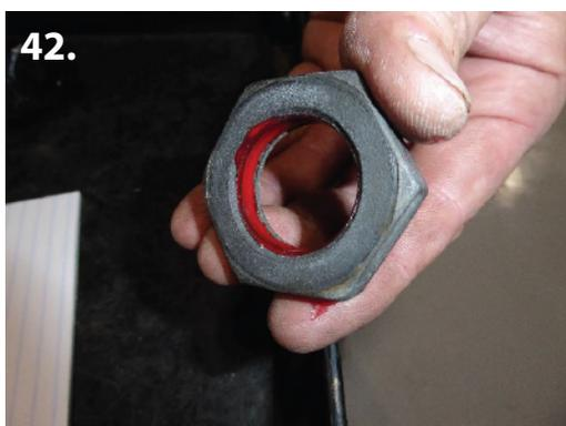
**39.** Before install new drop pitman arm, clean the factory splines and threads so there is no debris or oil. Be sure to clean the threads on the nut as well. Now apply the supplied red thread locker to the factory pitman retention nut and torque to factory specs. Make sure you install it the same way it came off the vehicle. Lining up the four alignment channels. (pic 42-43)
