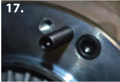
NOTE: Picture 16 shows in the **recommended** 20 degree position. You will need to install the McGaughy's transmission crossmember in this position. Picture 17 shows the 10 degree position, which can run the factory crossmember with trimming.
