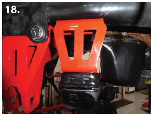
**18.** Clean the remaining weld material from the factory bump stop cup that was removed from the frame using an abrasive disc or flap wheel. Be sure to paint the bare metal.
