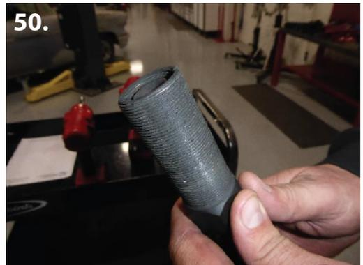
**44.** Once the drag link adjuster is removed, you must grind down flat the hexagon sides of the tie rod. Grind up to the threads. DO NOT grind any threads. When grinding the end of the tie rod, the goal is to extend the hexagon shaft right to the start of the threads. Making sure it is the same size from one end to the other. Be sure to stop right at the threads. You do not want to grind too much away. (pic 48-49)
