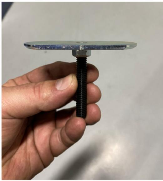
1. First apply loctite to the supplied retainer bolt. Then screw bolt into the retainer backing plate. Make sure bolt is flush with the top of the welded nut only. Do not screw the bolt past the backing plate.
