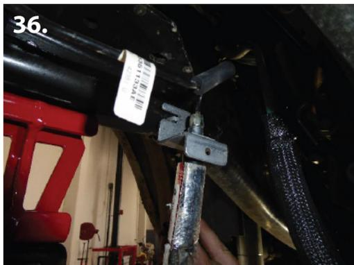
**35.** Redirect brake line, so that passenger side brake line bracket faces down instead of to the rear. (pic 36)
