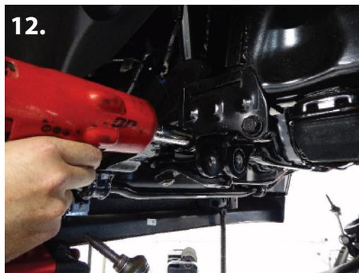
**13.** Unbolt the factory front track bar mount using a 21mm socket. (pic 11-12)
