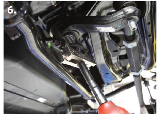
3. Remove the driver side drag link to pitman arm nut using a 21mm socket. Use a tie-rod removal tool to avoid damaging the factory tie-rod ends. (pic 4)
