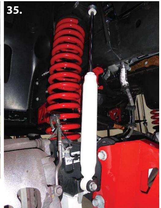
**33.** Install new lift coils. Be sure to use the factory coil isolators in the factory locations. The tighter winding face up and the more open windings face down. (pic 33-34)
