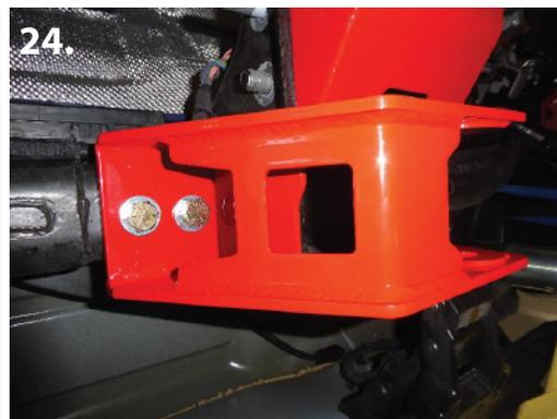
**25.** New radius arm drop dow brackets will slip over the outside of the original radius arm mount on the frame. Use the provided spacer and place it in between the original radius arm mount. Use the provided 18mm x 130mm bolt (pic 22)
