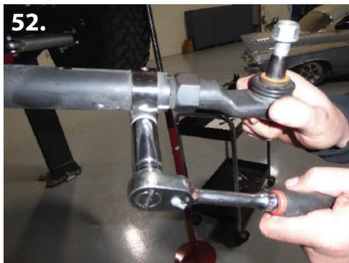
**46.** Now install the tie rod into the drag link with the tie rod facing up. (pic 51)
