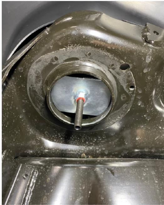
2. Next, insert the backing plate with bolt into the opening on the factory upper coil mount.
