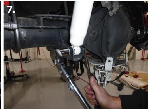
6. Remove the factory bump stops on both sides using a 15mm socket.
