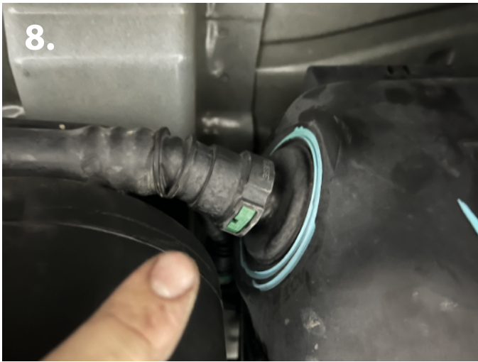
Disconnect fill line from def tank
