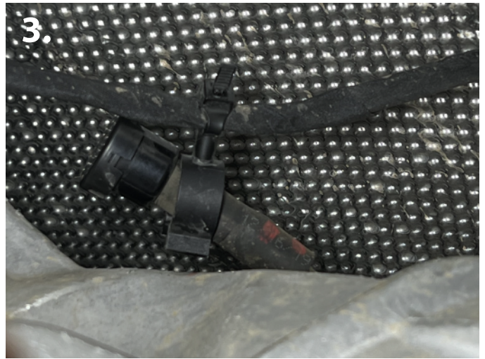
3. Disconnect solenoid wire clip on top of transfer case (same wire as pic 2, different clip)
