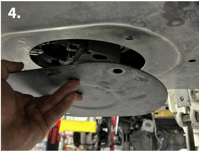
4. Remove access cover to get to def sending unit
