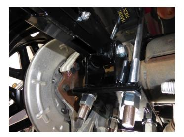
7. Now install provided bushings and sleeves in the traction bars.
