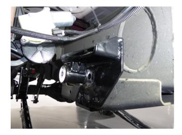
20. Be sure to use an impact wrench on the two upper frame bolts. This will ensure that the rivet nuts are secure.
