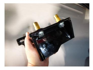
18. With both holes drilled out, insert the two provided 1/2" bolts into the frame bracket with the provided rivet nuts installed.19. Line up bracket with rivet nuts going into the hole drilled onto the frame.
