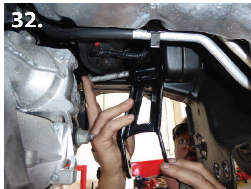
29. Use factory hardware in factory location to install driver side differential drop bracket. DO NOT TIGHTEN YET. (pic 30-31)
