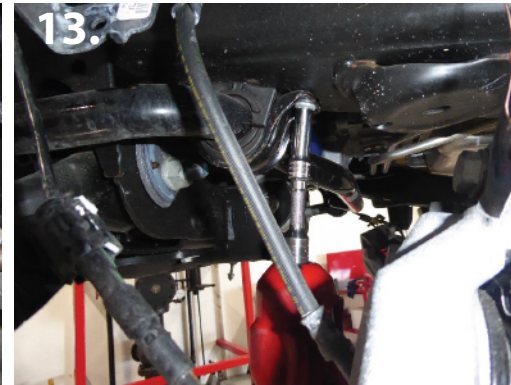
12. Use pry bar to remove CV axle. It will be tight because of the clip on the spline of CV axle. (pic 12) 13. Remove sway bar nut on lower mount of end link. (18mm) DO NOT remove upper nut of end link. Where end link is mounted to sway bar. 14. Remove sway bar mounts from frame. (10mm) (pic 13-14)
