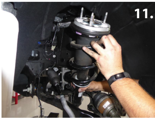
10. Remove lower bolt on factory strut. (15mm) (pic 10) 11. Remove factory struts. (pic 11)
