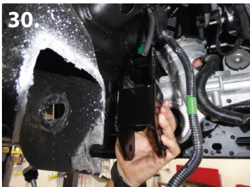
29. Use factory hardware in factory location to install driver side differential drop bracket. DO NOT TIGHTEN YET. (pic 30-31)
