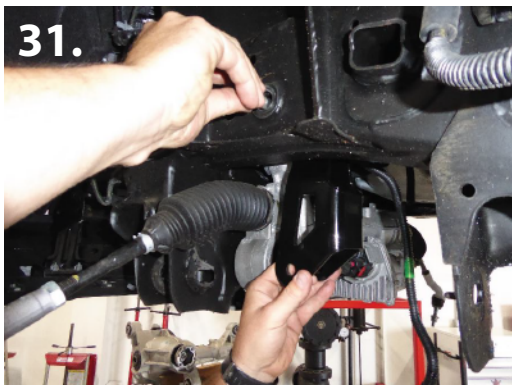
29. Use factory hardware in factory location to install driver side differential drop bracket. DO NOT TIGHTEN YET. (pic 30-31)
