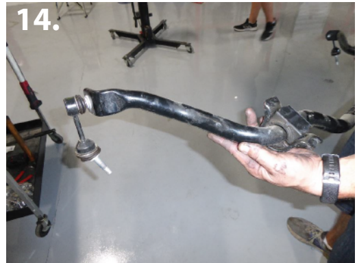
12. Use pry bar to remove CV axle. It will be tight because of the clip on the spline of CV axle. (pic 12) 13. Remove sway bar nut on lower mount of end link. (18mm) DO NOT remove upper nut of end link. Where end link is mounted to sway bar. 14. Remove sway bar mounts from frame. (10mm) (pic 13-14)
