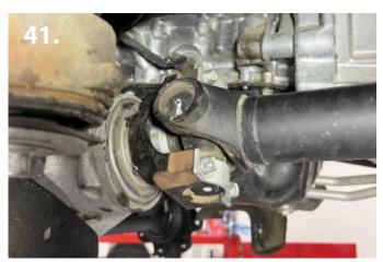
43. Reinstall the factory front drive line using the factory hardware. Be sure to use Loctite on all the bolts and torque to factory specs. (pic 41)
