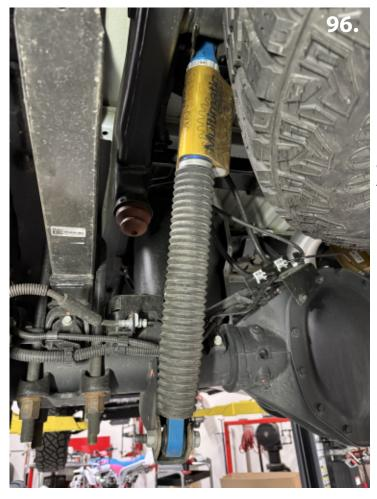
90. Now re-install the factory shocks. Shocks will install in the factory location using the factory hardware (pic 96).
