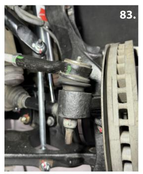
77. Install the new provided sway bar end links. New end links will now mount inside the lower a-arm. NOT on the outside like the factory ones were (pic 82).
