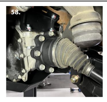
58. We recommend that you cut down the factory bump stop. We recommend that it be cut at the first rib (marked with the yellow dotted line) (pic 57).
