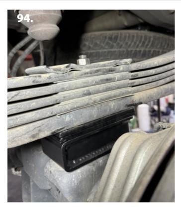
88. The provided center pin may be longer than you need. If so, you can trim the excess amount off. It is not neccessary to cut the pin though. (pics 93-94)
