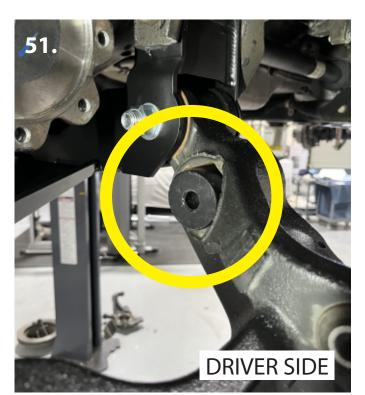
53. Insert the provided "NTD" (No Torsion Drop) puck spacer into the lower a-arm. Spacer fits inside where the factory torsion bar used to go (pic 51).
