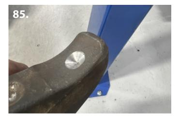
79. Before reinstalling torsion bars. Mark and drill a small indentation on the factory torsion key. This will keep the bolt from moving around on the key. Measure 1" from the end of key and mark the key in the center. Use a 5/8" drill
