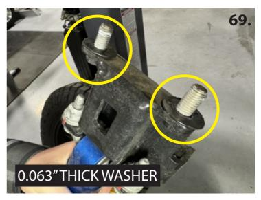
69. First you will install the AT4X shock brackets onto the vehicle in the factory shock location. Be sure to use the provided 16g washers on top of the bracket on the two studs. These washers MUST be used. (pic 68-69)
