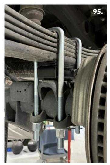
89. Now install the provided u-bolts (pic 95). Only snug the nuts. Do not tighten. Repeat the steps on the opposite side next. Once both sides are installed, then tighten up all the u-bolt nuts. Torque to 190 ft lbs.
