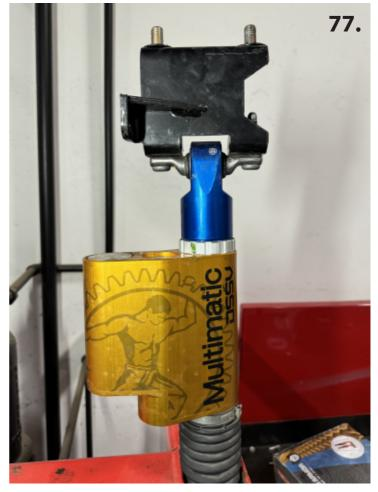
73. You can now install the shock bracket on to the factory AT4X shocks. Use the factory nuts and torque to the factory specs. Make sure you swap sides. Pic 76 and 77 are the same shock. This is the "new / now" passenger side shock. Pic 76 is the way you will see it on the vehicle. It is the side that faces out towards the tire. Pic 77 is the inside. It is the side that will face inside towards the engine. \*Please note: the Mulitimatic Logo will now face inside towards engine.
