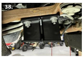
38. Install the driver side differential drop bracket using the supplied M12 x 30mm bolts, washers, and lock nuts. Snug bolts only. Do not fully tighten (pic 37).
