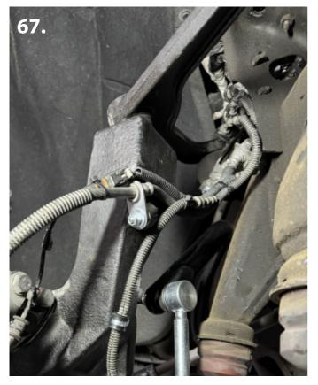
68. **THIS IS VERY IMPORTANT,** now that all the brake lines are in place and secure. Turn/rotate the spindle left to right fully. Make sure nothing is being over extended or stretched. Make sure nothing is rubbing or making contact with any part of the frame or suspension. You do not want any wires or hose to vibrate and be worn through. Make sure everything is in secure and in place 100% (pic 67).
