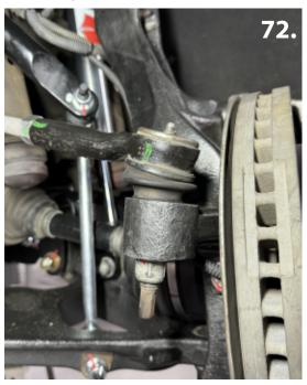
70. Install the new provided sway bar end links. New end links will now mount inside the lower a-arm. NOT on the outside like the factory ones were (pic 71).
