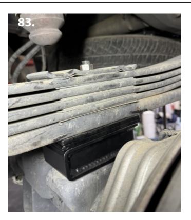
82. The provided center pin may be longer than you need. If so, you can trim the excess amount off. It is not neccessary to cut the pin though.
