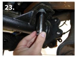
26. Remove the bolt on the driver side bottom front of the differential using 15mm socket. (pic 21)
