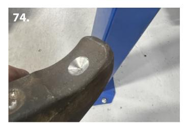
72. Before reinstalling torsion bars. Mark and drill a small indentation on the factory torsion key. This will keep the bolt from moving around on the key. Measure 1" from the end of key and mark the key in the center. Use a 5/8" drill
