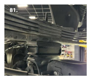
81. Remove clamps and place the provided lift blocks between leaf pack and rear end. Jack up rear end to keep blocks in place (pics 80-81). \*NOTE: pic 80 is the front of the lift block, pic 81 is the back side/rear of truck.
