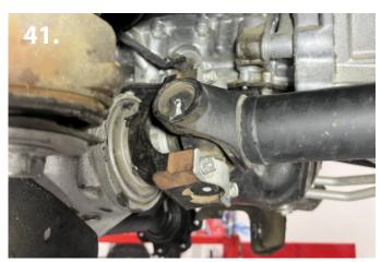
43. Reinstall the factory front drive line using the factory hardware. Be sure to use Loctite on all the bolts (pic 41).
