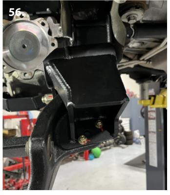
57. With both hole drilled, reinstall the NTD bracket on to the lower a-arm. Use the  $5/8" \times 6"$  GR8 bolt, washers, and nylon lock nut (pic 55). And  $5/16" \times 1-1/2"$  GR8 bolts, washers, and nylon lock nuts in the two holes that were drilled out on the lower a-arm (pic 56). Be sure to tighten the two 5/16" bolts first, then tighten the 5/8" bolt last.
