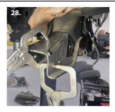
31. Next, bend template to curve on the driver side lower A-arm pocket where the new rear crossmember will mount (pic 27). Once bent over, clamp in to place (pic 28).
