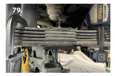
79. With the u-bolts removed, drop the rear end a small amount and clamp both sides of the leaf pack (pic 78). 80. With the leaf pack secure, remove the factory center pin. Install the provided rear shims on to the new supplied center pin and install on to the leaf pack. Torque to specs (pic 79).
