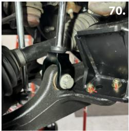
69. Now install the new front shocks in the factory location. Upper mount will use the provided  $1/2" \times 1-1/2"$  GR5 bolts, washers, and nuts. The lower mount will use the factory hardware. (pics 68-70).
