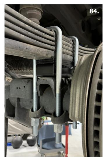
83. Now install the provided u-bolts (pic 84). Only snug the nuts. Do not tighten. Repeat the steps on the opposite side next. Once both sides are installed, then tighten up all the u-bolt nuts. Torque to 190 ft lbs.
