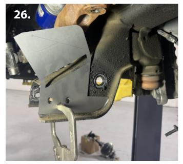
30. Start on the driver side (pic 24). Line up the supplied cut-off template holes to the factory holesand clamp in to place (pic 26).
