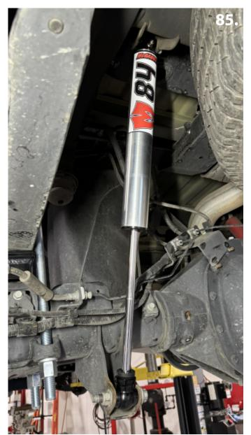
84. Now install the new lift shocks. Shocks will install in the factory location using the factory hardware (pic 85).
