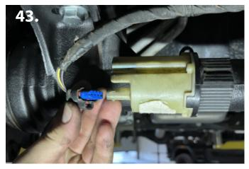
44. Install the supplied vent line extension on top of the differential housing. Then attach the factory vent line to the new extension using the supplied fitting (pic 42). 45. Reconnect plug on passenger side of differential (pic 43).
