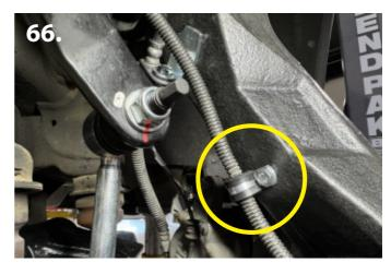
66. Next, install the brake line extender bracket on to the new lift spindles. Driver side and passenger side brackets are different (driver side shown). Connect the extender bracket to the spindle in the existing hole on the back. Use the supplied M6 x 10mm bolt on the back of spindle. Then, install the factory bracket to the new extender using the provided  $1/4" \times 3/4"$  bolt, washers, and nut (pic 65).
