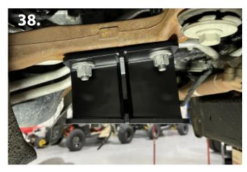
38. Install the driver side differential drop bracket using the supplied M12 x 30mm bolts and washers. Snug bolts only. Do not fully tighten (pic 37).
