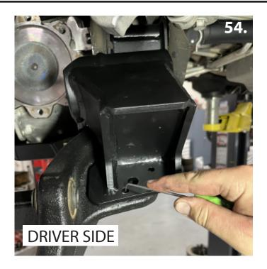
54. Now install the NTD bracket on to the lower a-arm. NTD bracket will slide over the install puck spacer. Use the 5/8" x 6" GR8 bolt. Bolt will go through the puck spacer on the lower a-arm (pics 52-53).
