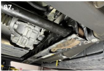
80. Re-install the torsion bars in to the new location in the NTD brackets on the lower a-arms. Be sure to install the torsion bars the exact same way they came out of the truck. Do not swap sides or turn around. You may have to lift up on the lower a-arm so that the torsion bar can pass through the NTD brackets easier (pic 86-87).
