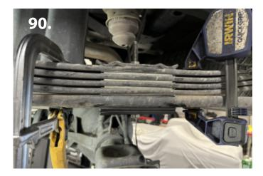
85. With the u-bolts removed, drop the rear end a small amount and clamp both sides of the leaf pack (pic 89). 86. With the leaf pack secure, remove the factory center pin. Install the provided rear shims on to the new supplied center pin and install on to the leaf pack. Torque to specs (pic 90).
