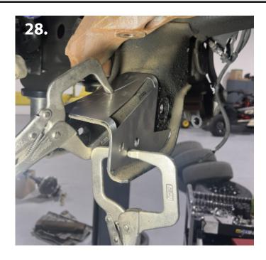
31. Next, bend template to curve on the driver side lower A-arm pocket where the new rear crossmember will mount (pic 27). Once bent over, clamp in to place (pic 28).
