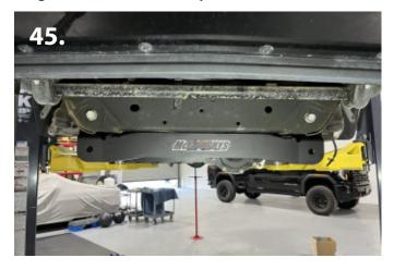
47. Install the front crossmember in the original lower a-arm location, using the factory lower a-arm hardware (pic 45). Snug only, do not fully tighten bolts.
