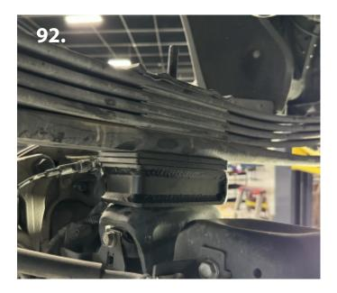
87. Remove clamps and place the provided lift blocks between leaf pack and rear end. Jack up rear end to keep blocks in place (pics 91-92). \*NOTE: pic 91 is the front of the lift block, pic 92 is the back side/rear of truck.
