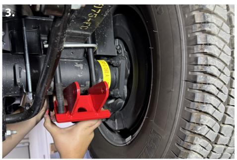
4. Install new provided lower u-bolt plate. Make sure the mounting tabs are facing forward towards the front of the vehicle. \*The mounting plate radius is specific for your application. Make sure the bracket radius is tight and no gaps on your rear end. If your bracket is not the same radius as your axle, DO NOT continue. Contact us immediately.
