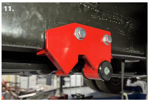
16. To make this next step easier, remove the frame mount from the shackle mount. Bolt the frame mount onto the frame using the provided hardware into the two rivit nuts you just installed. (pic 11)
